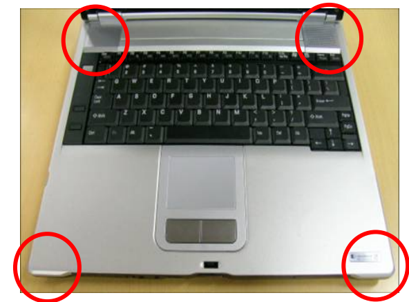
Extended corners are a key part of the Shock Protection Design concept and provide more space for shock absorption.
