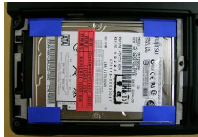
Rubber tabs encase the hard disk drive for maximum protection. This is a key part of the Toshiba Shock Protection Design,
